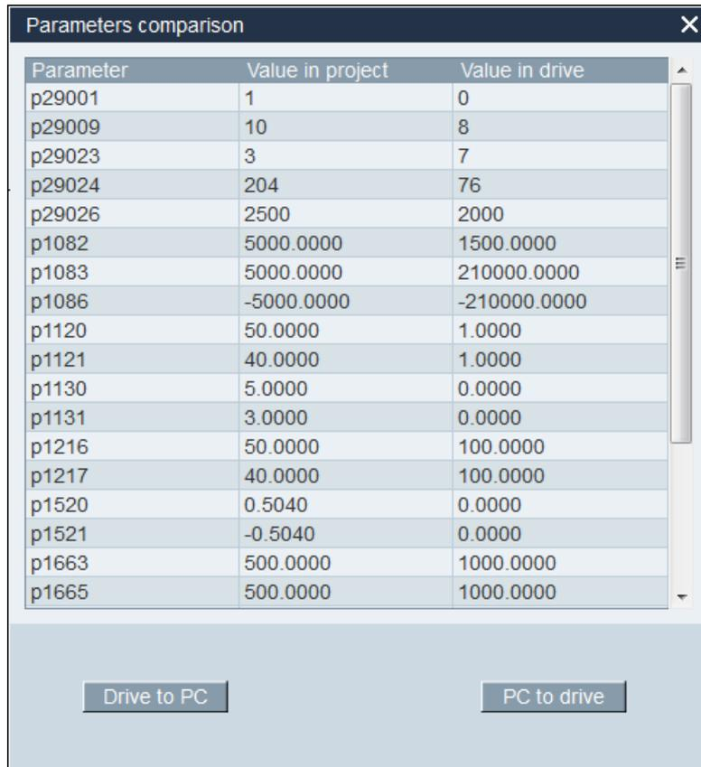
The image shows a dialog box titled "Parameters comparison" with a close button (X) in the top right corner. It contains a table with three columns: "Parameter", "Value in project", and "Value in drive". The table lists 20 parameters with their respective values. Below the table are two buttons: "Drive to PC" and "PC to drive".
