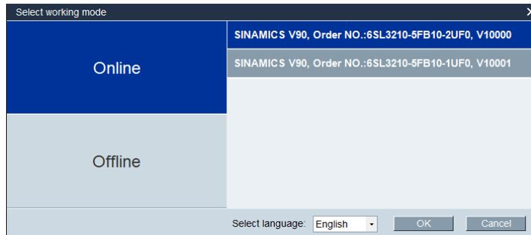
Select the target drive type, and click **OK** to establish communication between SINAMICS V-ASSISTANT and the drive. SINAMICS V-ASSISTANT reads all parameter settings from the connected drive and the main window displays the drive information on the following panel:
